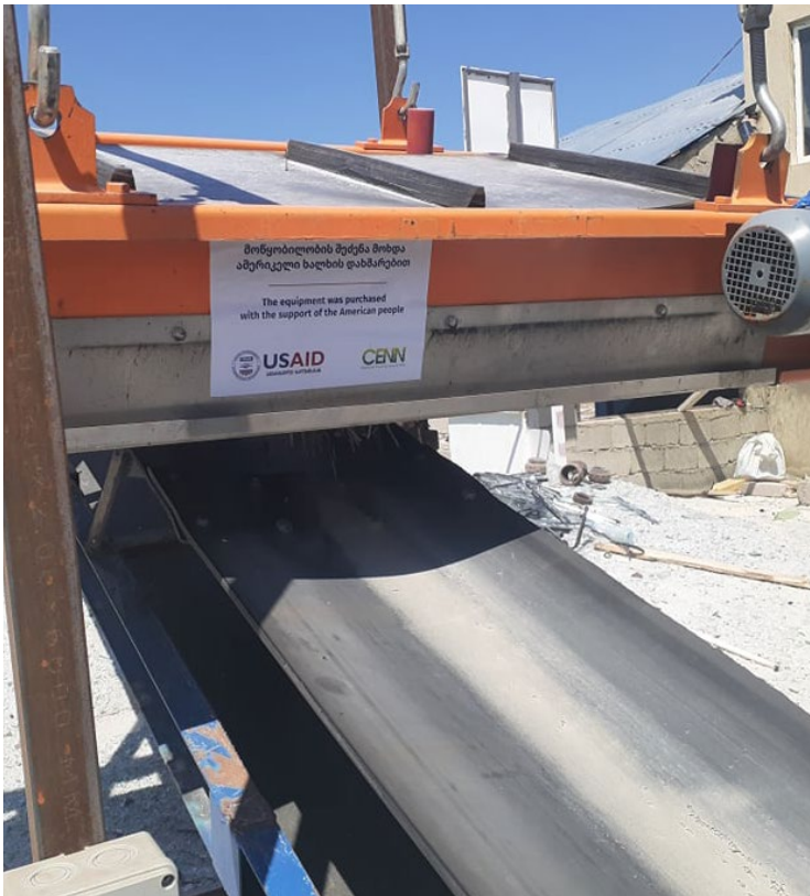
Conveyer belt with Vibro-Flume to ensure the efficient and high-quality treatment process of glass waste.
